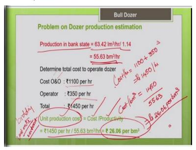
Already it is given to you the ownership and the operating cost is 1100 per hour, operator cost is given. So, cost per hour = 1100 + 350 rupees, so that gives you 1450 rupees per hour is the hourly cost. So, now let me calculate the cost per bank meter cube, it is nothing but the hourly cost by hourly productivity. So, 1450 divided by hourly productivity is 55.63, so this gives me the answer as rupees 26.06 per bank meter cube.
