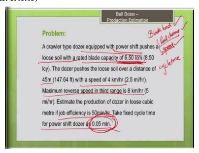
So, you know the haul distance and speed, so you can calculate the cycle time. So, based on using this input parameters, I can estimate the productivity of the bulldozer. So, let us see how it is done.
