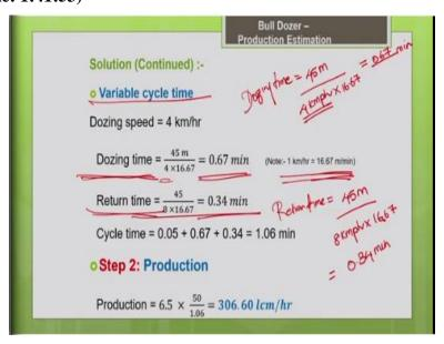
So, variable cycle time is nothing but it is made up of dozing time and the return time, onward journey, return journey. So, dozing time you know the dozing distance 45 meter and the speed is
