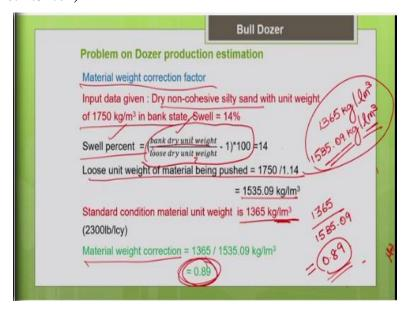
So, now you can compare both, your standard condition is 1365 kg per loose meter cube. So, now your project condition is 1,535.09, per loose meter cube. So, obviously your project soil is more denser than compared to the standard condition curve. So, that means, this is going to affect your productivity when the soil is more denser, it is going to be difficult for the bulldozer to push it. So, that is definitely going to reduce the productivity.
