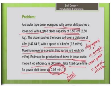
Now let us workout another problem a different approach of estimation of the productivity. So, in this a crawler type bulldozer is given, this equipped with power shift mode. So, automatic gear change, it pushes a loose soil with blade capacity 6.5 loose cubic meter. So, the blade capacity is given to you 6.5 loose cubic meter, and the dozer pushes the loose soil over a distance of 45 meters.
