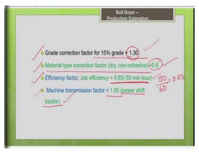
Grade correction, you are moving down the slope -15%. So, your correction factor increases, it is going to enhance the productivity. So, from grade perspective, it is better than the value taken from the ideal curve. Then material type, here it is non-cohesive silty sand, so obviously it will affect the productivity correction factor is less than 1, 0.8. Job efficiency, machine is working for 50 minutes in a hour, so accordingly 50 divided by 60, find the correction factor it is 0.83.
