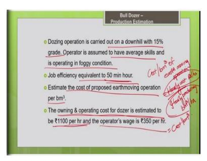
Then other things like operator the curve was drawn for excellent operator skill. So, in our problem the operator skill is average. So, accordingly you have to choose the correction factor and apply. So, your correction factor is going to be less than 1, because it is average is going to reduce your productivity. Similarly, the material type, material type is non-cohesive silty sand, so that will definitely reduce the productivity.
