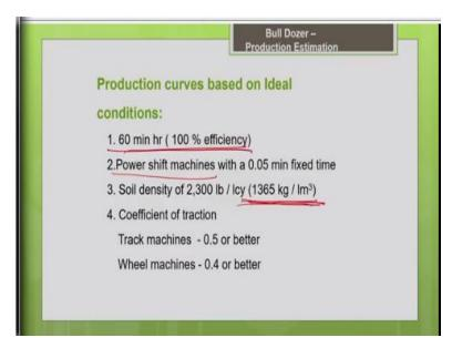
And hope you remember these curves are valid only for these ideal conditions. So, 60 minutes hour but in your project in this problem we found that the machine is working for 50 minutes an hour. So, you are supposed to apply the job efficiency, you have to apply the correction factor accordingly. So, this curve is applicable for power shift mode, automatic usage. So, in this problem also you have the automatic gear change, so no need to apply the correction factor.
