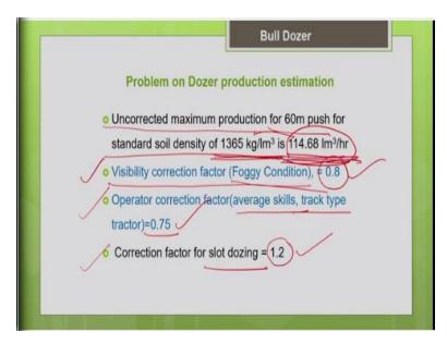
Let us workout the solution for this problem. As I told you the first step is we need to find the uncorrected maximum production for the 60-meter push distance for the standard soil density of 1365 kg per meter cube. So, how will you find the production? So, using the production curves as I told you using this production curve for your model and for the dozing distance, what is the value we can take it, this is called as the uncorrected value.
