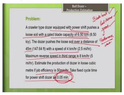
So, you know the blade capacity, you know the blade load, that is known. So, you know the haul distance the dozing distance is known, so it is known, you know the speed of the machine. If the speed is not given in that case you have to go for the performance chart, with the help of performance chart you have to find the speed. But in this problem speed is given to you directly.
