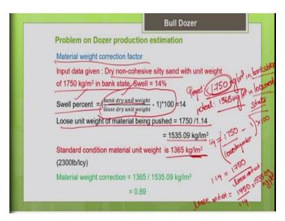
Now another important correction factor which we are yet to determine is material weight correction factor. As I told you in this project we are going to deal with non-cohesive silty sand. It is unit weight is given as 1750 kg per meter cube in bank state; it is 1750 kg per meter cube in bank state, so this is your actual project. But the curve value what we have chosen, productivity value what we chosen is for the ideal condition where the soil density is 1365 kg per meter cube.
